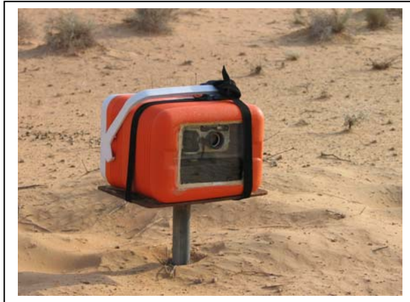
Pictures 1 & 2 , showing on the left the modified coolbox forming a housing for the receiver and the camera kit. Straps are used to secure the housing to a base pole. On the right the transmitter is housed in a PVC box and fixed to a pole.
