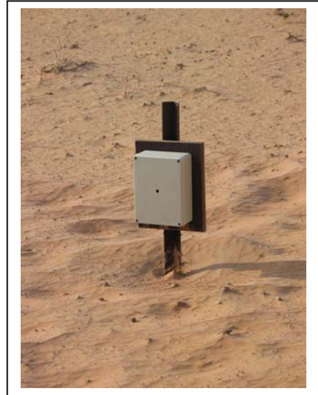
Pictures 1 & 2 , showing on the left the modified coolbox forming a housing for the receiver and the camera kit. Straps are used to secure the housing to a base pole. On the right the transmitter is housed in a PVC box and fixed to a pole.
